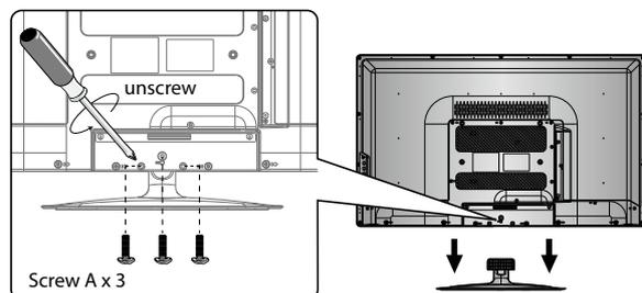
2. Mounting on the wall. This TV is designed to be wall-mounted with a standard 200 mm x 100 mm mounting kit (sold separately) designed for flat-panel TVs. Mount this TV according to the instructions included in the mounting kit. Due to space restrictions, we recommend that you make all connections (refer to page 15-18 and page 45 for details) before mounting on to the wall.
