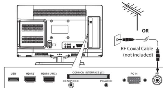
Connect one end of the RF coaxial cable to the aerial socket on the wall and the other end of the cable to the RF (75Ω) socket at the rear right side of your TV.
